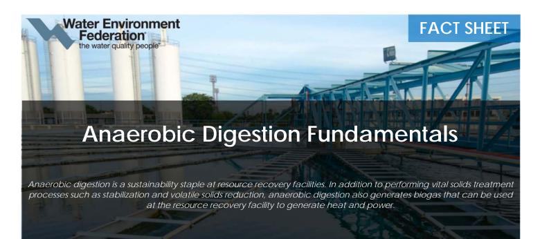
Anaerobic digestion is a solids stabilization process commonly used at municipal and industrial water resource recovery facilities (WRRFs). The primary objective of anaerobic digestion is to convert the microbiological cells and other solids generated during the treatment process to a stable end product. Other solids stabilization processes include aerobic digestion, composting, thermal drying, thermal oxidation, and alkaline stabilization.
