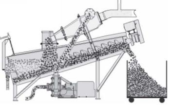
Figure 5: Cyclone and Classifier (Wemco, Inc.)
